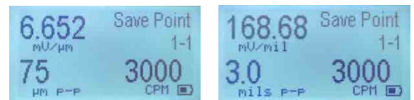
Model 9110D Portable Vibration Calibrator discovers a proximity probe cabling error despite correct gap voltage
